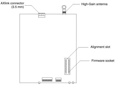
FIG. 8 AXR-NWS circuit board and IC socket location
